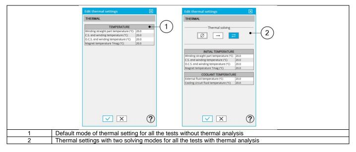
In the current version, the tests which allow using the thermal solving mode are the computations of working points defined by I,  $\Psi$ , N with motor or generator convention for Synchronous Machines with Permanent Magnets with inner rotor only.
