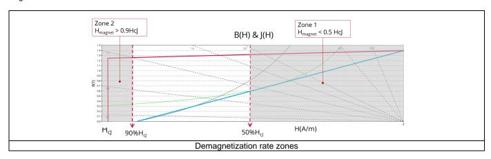
During the analysis of the machine behavior over one electrical period, sensors compute the levels of magnetic fields in all the magnets. The **Demag. Rate** (demagnetization rate) < CF50 (in % or P.U.) gives the percentage of magnet area where the maximum computed magnetic field is below fifty percent of intrinsic coercivity (HcJ). It corresponds to the area of magnet in Zone 1
