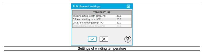
It is possible to define temperature of the three main parts of the stator winding:
