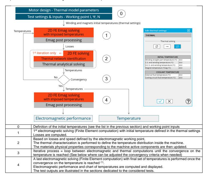
(1) The temperatures which are considered for computing the final machine performance (step 4 in the previous flow chart) can be read in the table dealing with "Winding and Magnet characteristics" of the test configuration at the beginning of result report. See below illustration.
