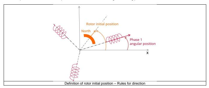
The winding axis of the reference phase is defined from the phase shift of the first electrical harmonic of the magneto motive force (M.M.F.).
