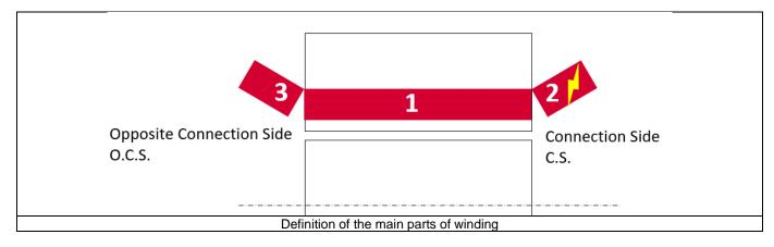
The resulting resistance of each part of the winding is computed as: Winding straight part resistance (part 1) Connection Side (C.S.) end winding resistance (part 2) Opposite Connection Side (O.C.S.) end winding resistance (part 3)
