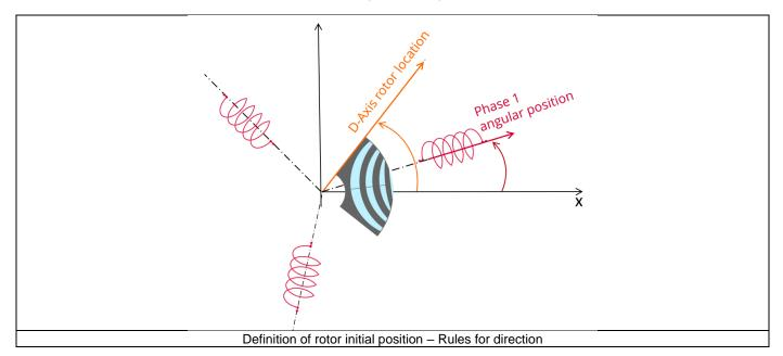
The winding axis of the reference phase is defined from the phase shift of the first electrical harmonic of the magneto motive force (M.M.F.).
