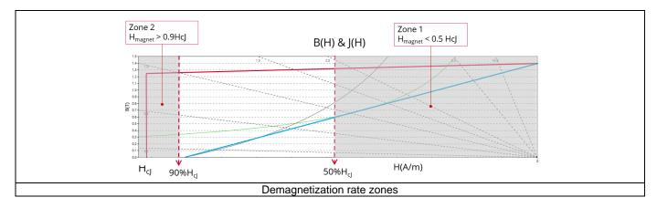
During the analysis of the machine behavior over one electrical period, sensors compute the levels of magnetic fields in all the magnets. The **Demag. Rate** (demagnetization rate) < CF50 (in % or P.U.) gives the percentage of magnet area where the maximum computed magnetic field is below fifty percent of intrinsic coercivity (HcJ). It corresponds to the area of magnet in Zone 1
