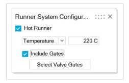
You can also define valve gates for the hot runners to control the flow of material through the gates. Click **Select Valve Gates** on the Runner System Configuration window and use the microdialog options to define the injection controls. Click **Add Controller** to specify when a valve opens or closes during the injection stage based on time, pressure, flow front or volume. Controls for multiple gates must be set up separately for each gate.
