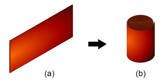
Figure 1: A thin metallic sheet (a) folded in the shape of a foil coil (b).
