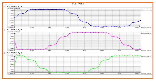
The goal is to note the positive zero crossing voltage position for each voltage
