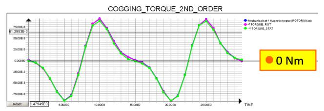
The use of a  $1^{st}$  order mesh line leads to obtain better results than the use of a  $2^{nd}$  order mesh point. Plus we have a 20% decrease of the computation time.
