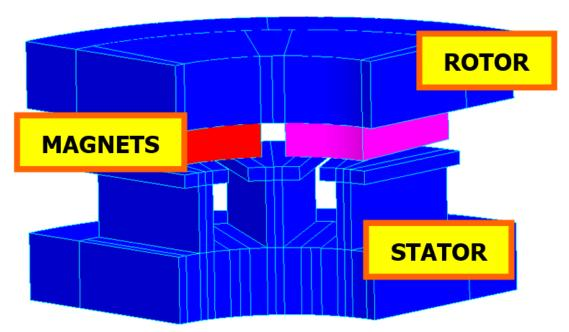
Performances of the motor are computed using the transient magnetic 3D application. A circuit coupling is not needed in this case.
