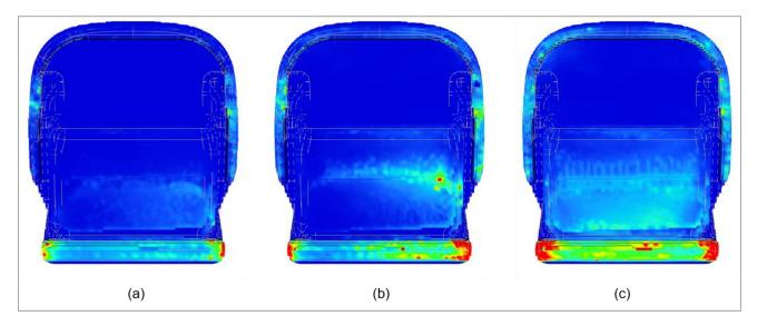
• Shrinkage defect modulus: This result type predicts volume shrinkage of the foam, which occurs if the foam is too soft even after demolding. It depends on the demolding time, pouring mass, mold temperature, and reaction rate, and can only be used on flexible polyurethane foam.
